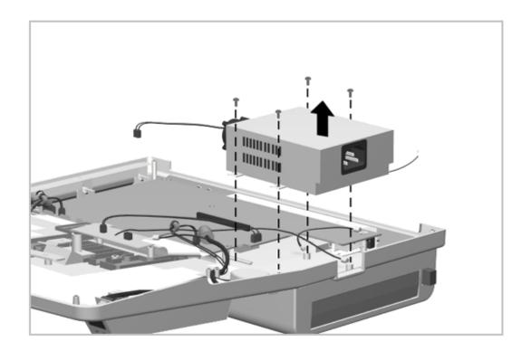
Figure 6-13. Removing the Power Supply Screws and Power Supply To install the power supply, reverse the procedure presented above. Be sure to reconnect the ground wire.
